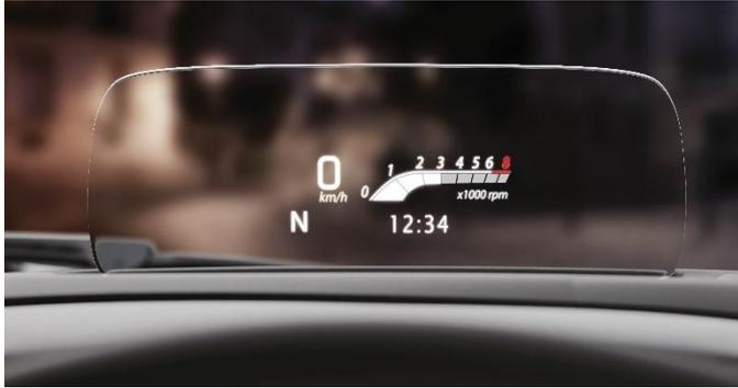
To make urban cruising more futuristic, safe, convenient and drive up the 'wow' factor, the New Age Baleno comes with a state-of-the-art first in its segment colored Head Up Display. It allows customers to drive without taking eyes off the road by displaying critical information like speed, RPM, fuel economy, and other pertinent notifications in a way that does not disturb the attention of the driver from the road.
